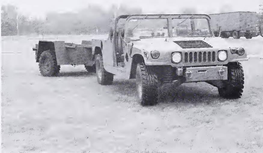
Three-quarter view of the Desert Mobility Vehicle System (DMVS) — TACOM-modified HMMWV and fabricated trailer.
